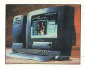
end Infinia 7260 (\$2899) has a 266-MHz Pentium II processor, a 6.4-GB hard drive, and 64 MB of EDO DRAM. All systems offer one-touch Internet access: A button mounted on the monitor gives you access to e-mail and special-interest Web sites through a Web service that Toshiba provides.
